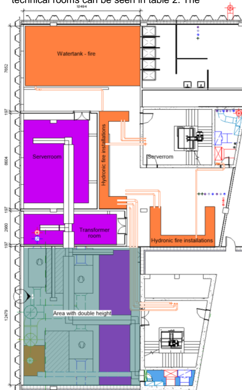
Figure 19: Floorplan over the technical room at level -1
