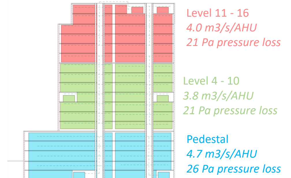
Figure 9: Showing the division of zone types for the AHUs indicated by colours. There are two AHUs within each zone. One unit's ventilation rate and pressure loss to the farthest air terminal is indicated to the right.
